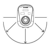
The installation height is between 140 and 160 cm (floor to bottom edge of housing).
