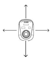
The installation surface measures at least 262 x 222 mm (height x width).
