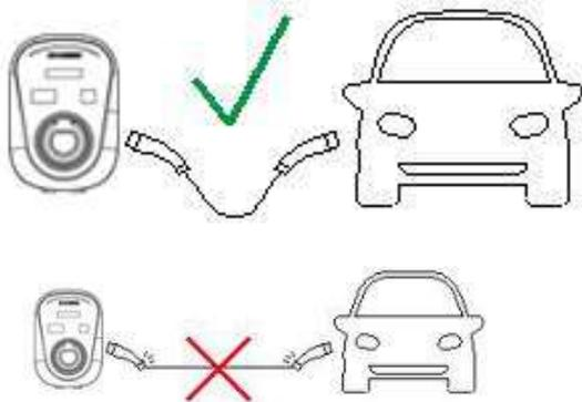
The charging cable must not be under strain, during the charging process.
