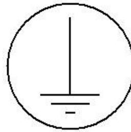
Charging station must be connected to a protective earth conductor
