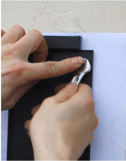
5. Tighten the top screws with a wrench.
