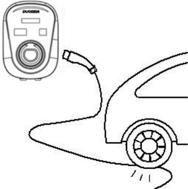
The charging cable and the charging connector must not be driven over.
