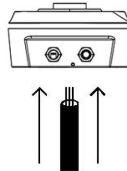
1. Ideally, the cable entry is from the underside of the housing base
