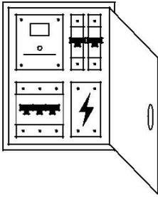
The power supply in the domestic power distribution box must be protected separately by a suitable and accurate dimension miniature circuit breaker (C characteristic)
